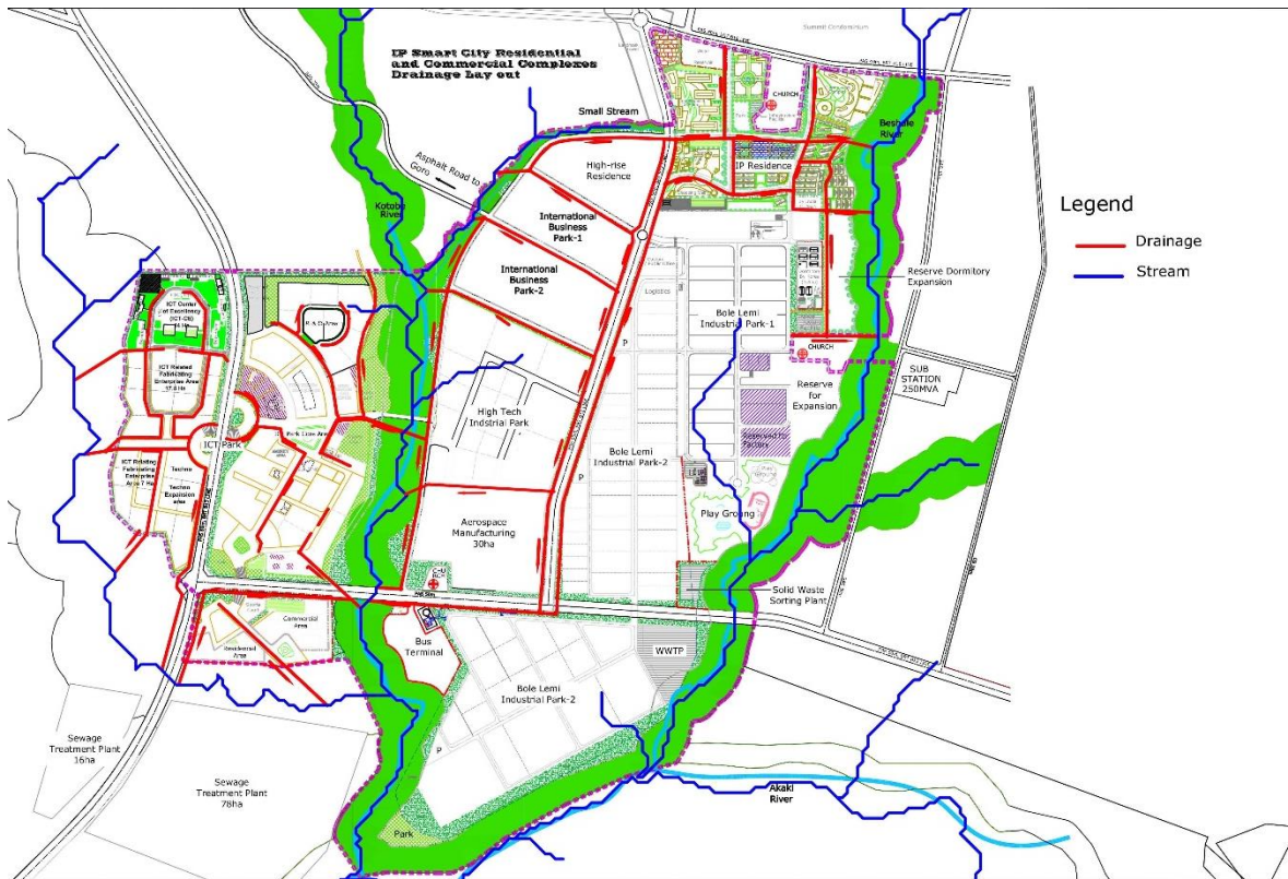
Map 23: Proposed Drainage Layout
