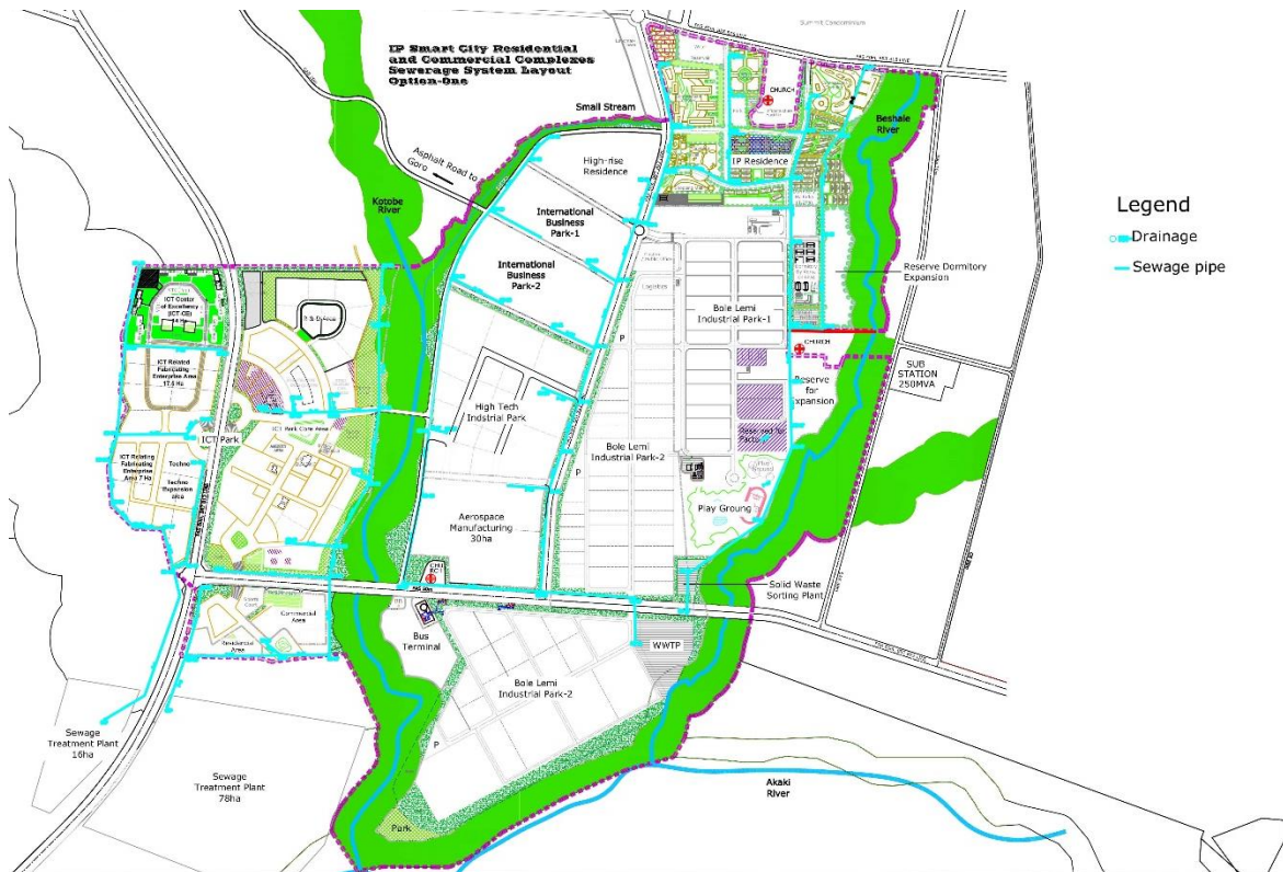
Map 24: Proposed Sewer Layout (Option I)
