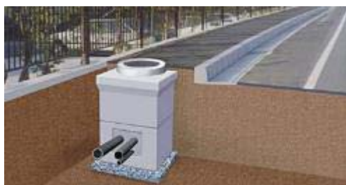
Figure 3.5.7: Example of Precast Manholes
