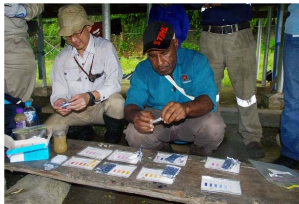
Photo 11: Water testing using the PACKTEST at site
