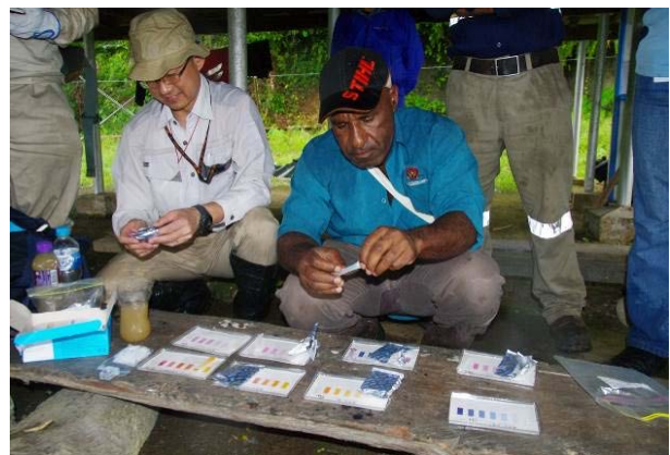
Photo 11: Water testing using the PACKTEST at site
