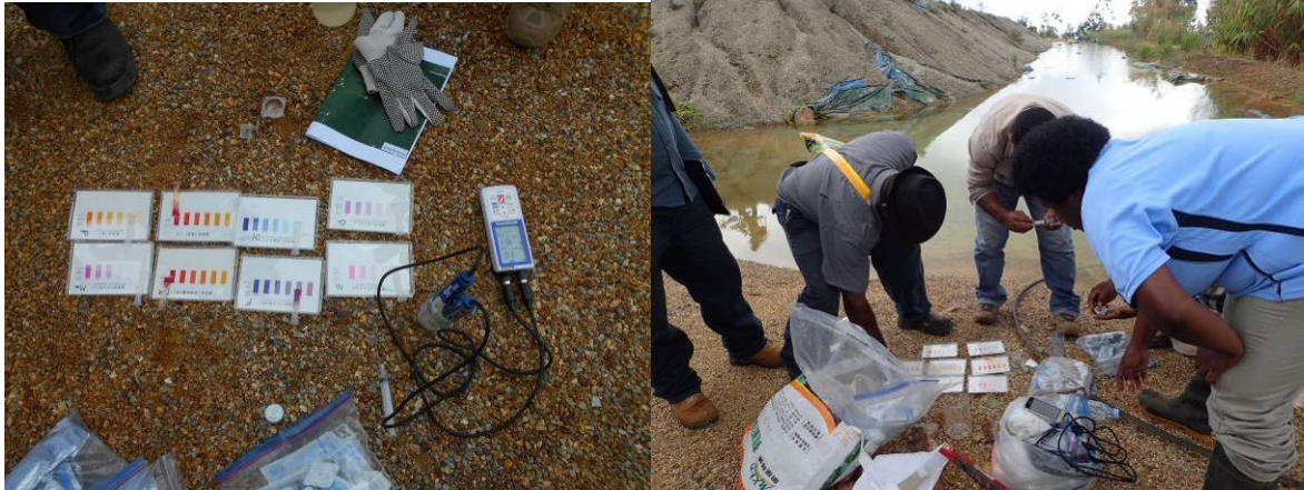
Photo. 9: Quick spot measurements by using the Pack Test
