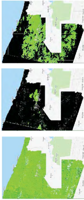
Figure 3.7 The cloud-free image for a weekly image from 2018-01-28 to 2018-02-04 (black-colored areas are masked cloud and/or shadow areas) derived by using the greenest-pixel method (left), the QA band method (center), and the cloud-shadow masking method (right).
