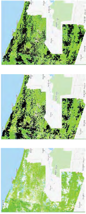
Figure 3.4 The cloud-free image of 2015 (black-colored areas are masked cloud and/or shadow areas) derived by using the greenest-pixel method (left), the QA band method (center), and the cloud-shadow masking method (right).
