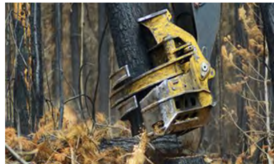
Figure 3-3-5: Harvesting neck used to facilitate directional felling (Tiger Cat website)
