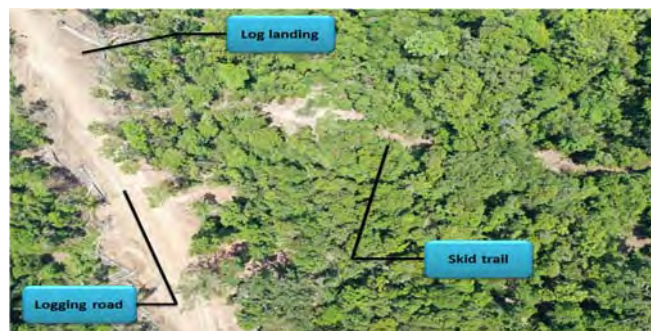
Figure 9: Visualization of skidding trails from drone is not always continuous
