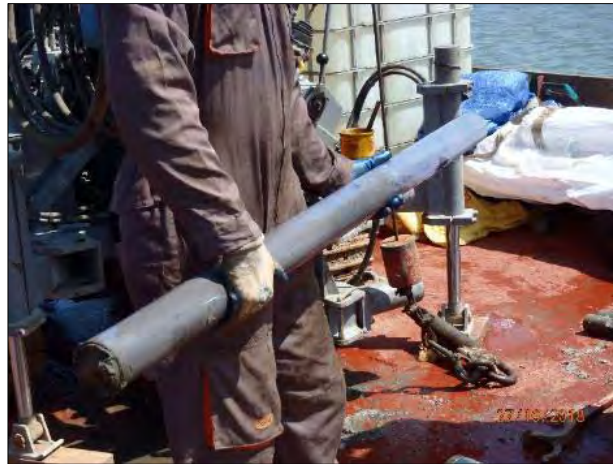
Photography 18 : Recovery of samples in the carrot
