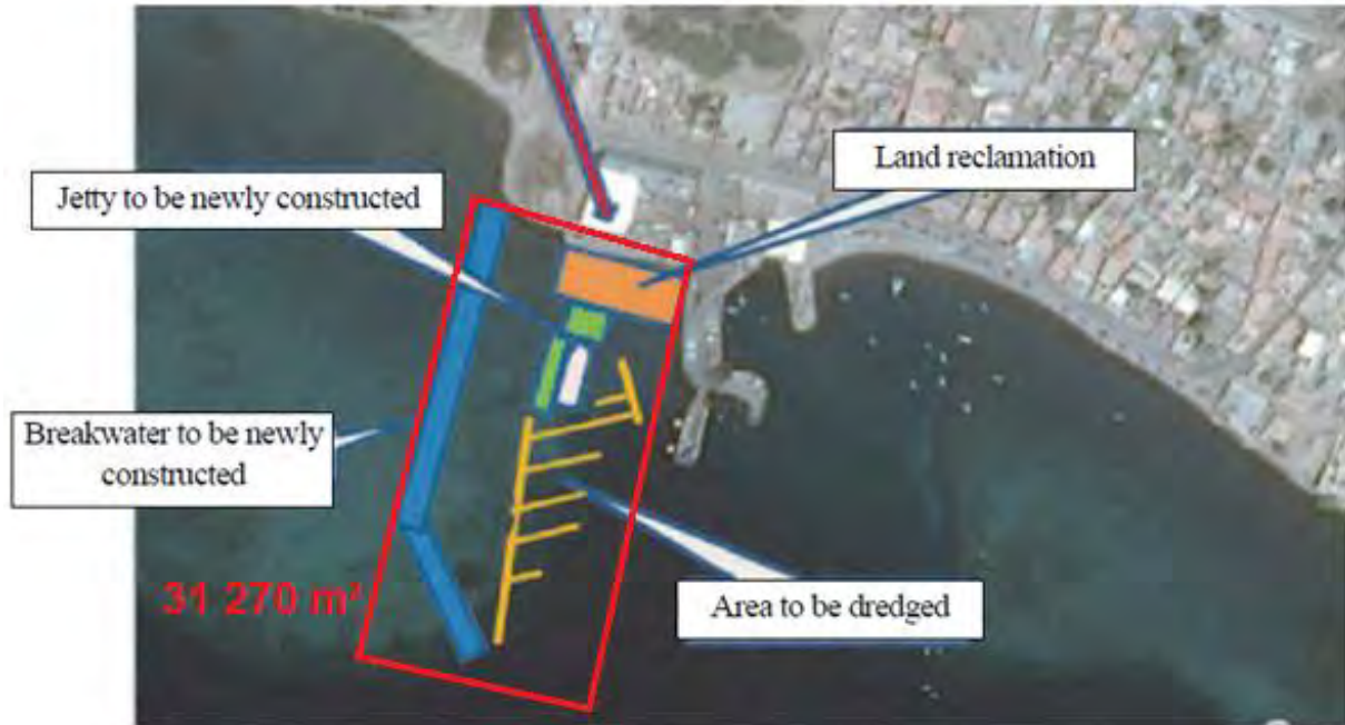
Figure 13 : Map showing Project area (red rectangle), planned area for breakwater (blue thick line), Land reclamation (orange rectangle), Jetty (green) and dredging area (yellow)
