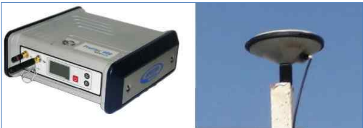
Figure 10 : Proflex 800 receiver(left) and associated GNSS antenna fixed on the pole
