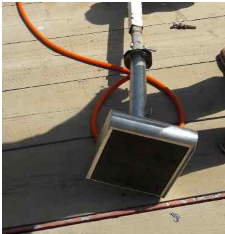
Figure 15 : SBP transducer fixed on pole
