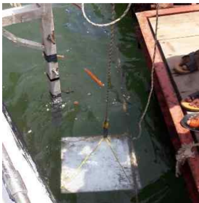
Figure 8 : Metal plate used for PA500 calibration
