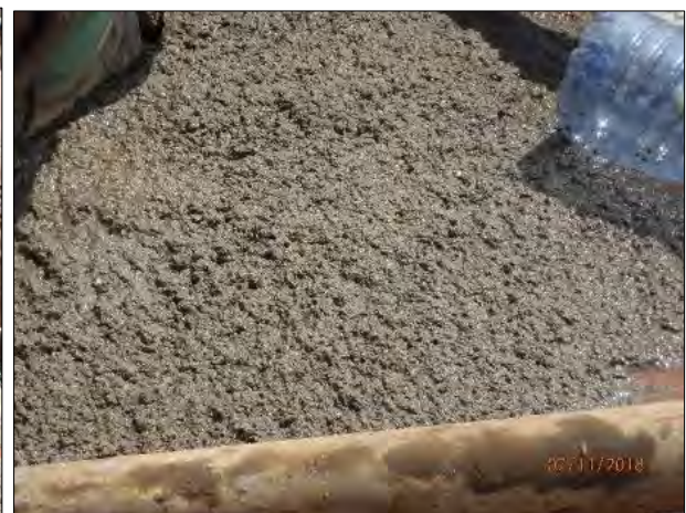
Photography 16: Sediments out of tubing during carotage
