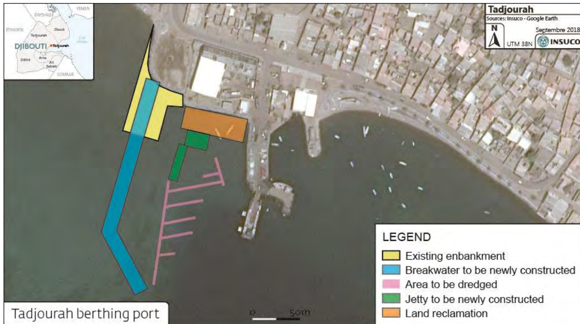
Figure 2: Existing and new infrastructures to be built in the port of Tadjourah
