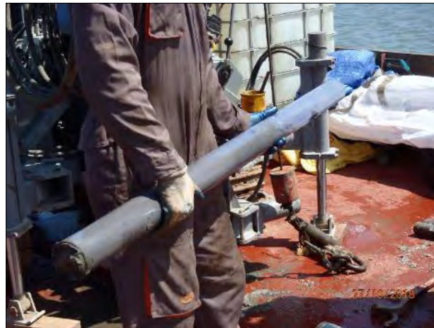
Photography 18 : Recovery of samples in the carrot
