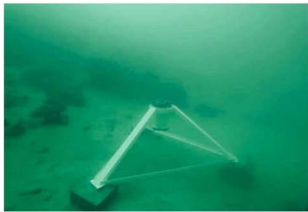
Wave Observation at Tadjourah Port Natural condition survey: Wave observation (Tadjourah Port)
