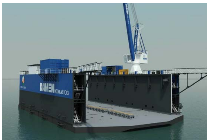
Figure 3.2-5 Schematic view of the floating dock (DAMEN brochure)
