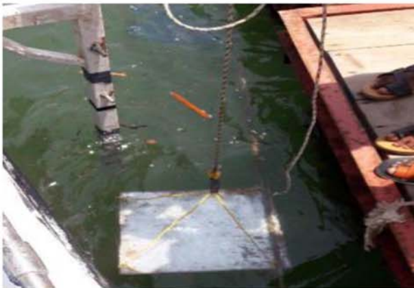
Bathymetric survey (Calibration) at Djibouti Port Natural condition survey: Bathymetric survey (Djibouti Port and Tadjourah Port)
