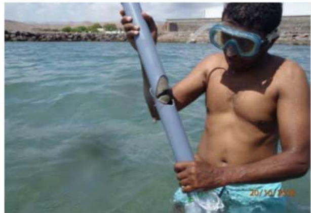
Sampling seabed sediment at Tadjourah Port Environmental survey: Sampling seabed sediment (Djibouti Port and Tadjourah Port)
