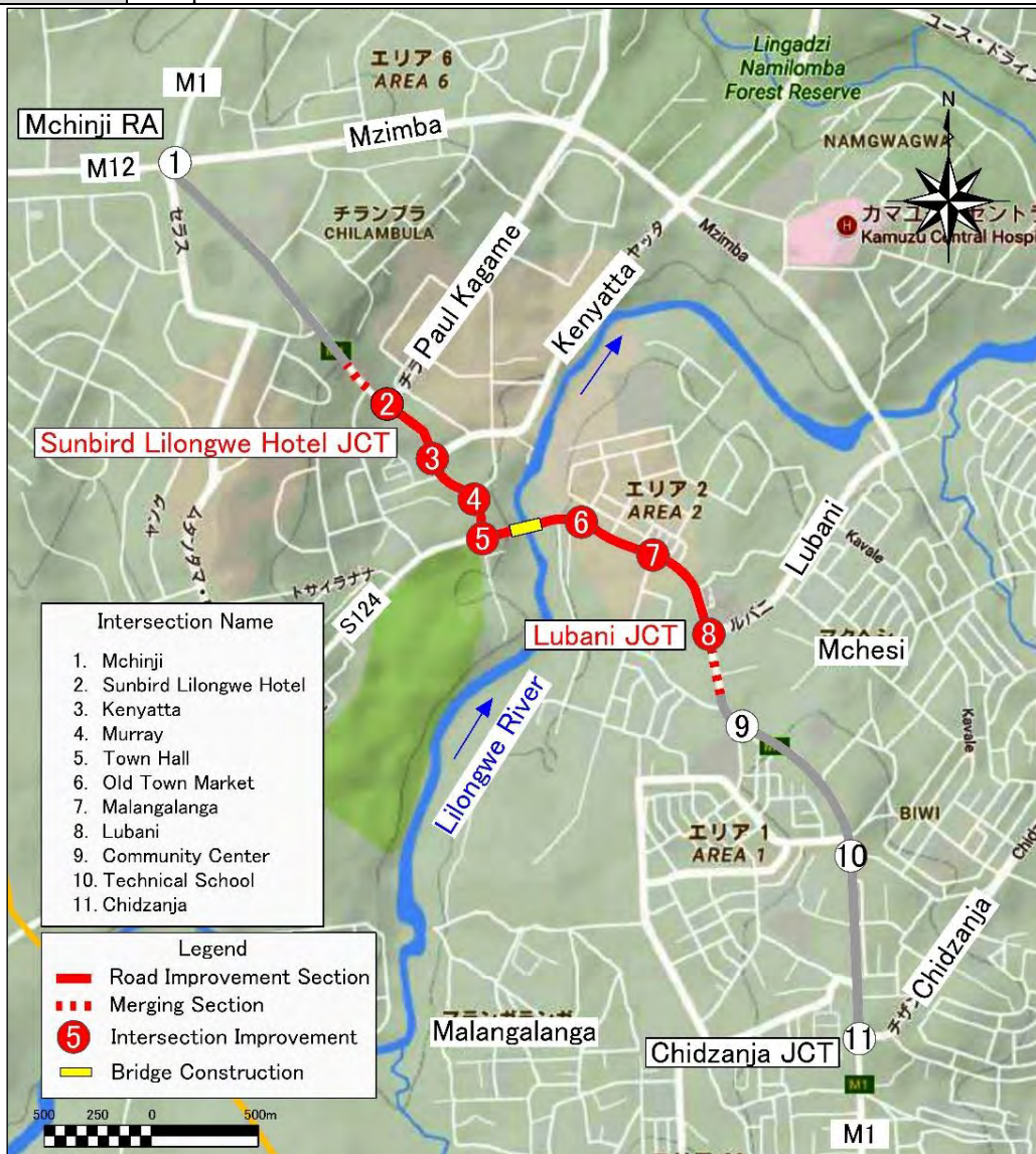
Figure 2-2-1 Scope of the Project
