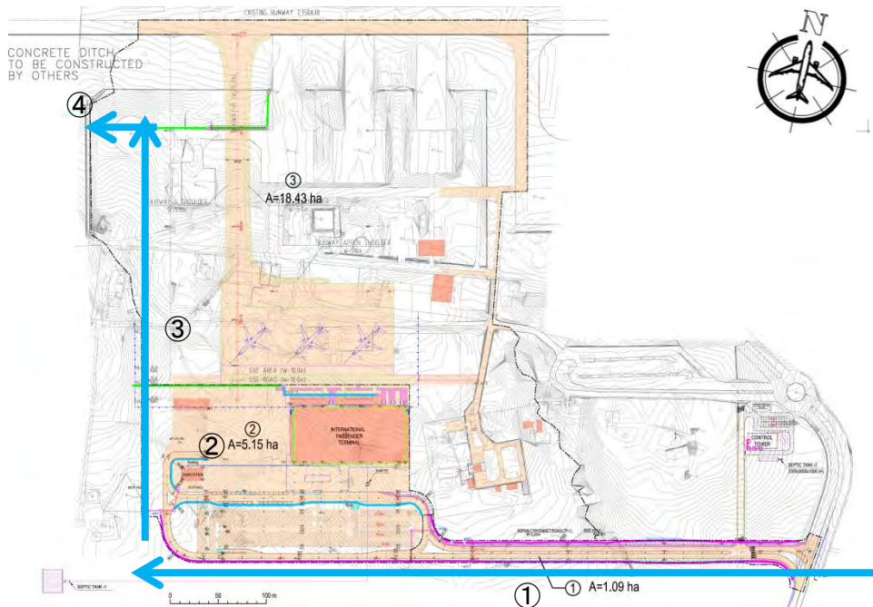
Figure 2.2.2-26 Drainage Catchment Area
