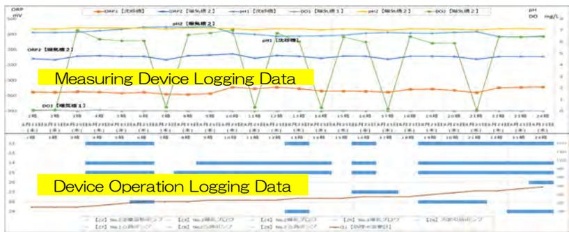
By comparing Measuring Device Logging Data and Device Operation Logging Data in time series, it can be confirmed that treatment is done in properly. Get correlation by comparing each parameters of Measuring Device Logging Data.
