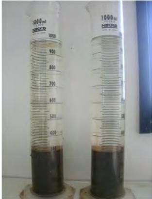
The sedimentation of sludge is good, and the separated supernatant water is also clear.
