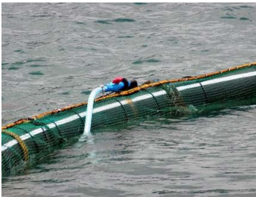
Submerging the cage with plastic nozzle
