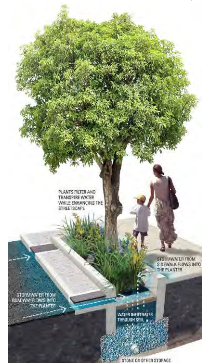
Figure 4.1.2 Example of Stormwater Planter
