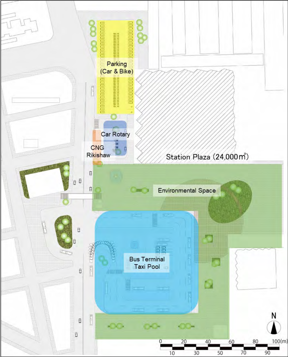
Figure 3.5.5 Example of Facility Layout for Large Station Plaza
