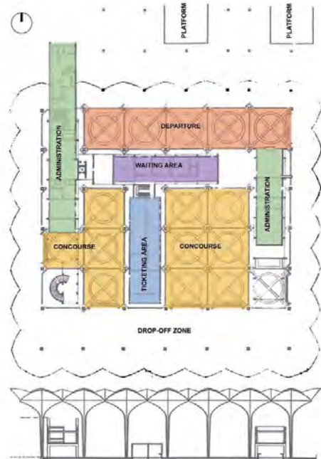
Figure 9: Plan and elevation of Kamalapur railway station
