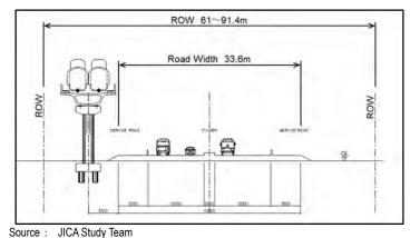
Figure 4.1.3 Typical Cross Section of the Alignment Parallel to Road
