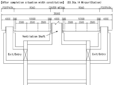
Figure 4.2.41 Road width after the Construction of Mirpur 14 Station (Plan)
