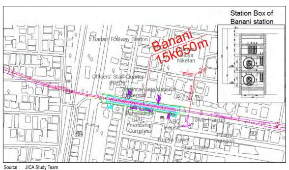
Figure 4.1.8 Horizontal Alignment before and after Banani Station
