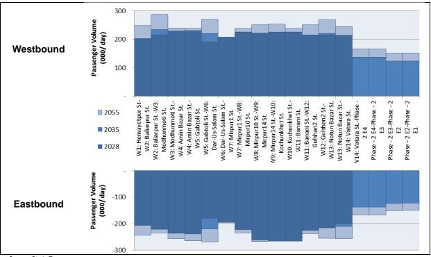
Figure 3.4.10 Line Volume by Section of MRT Line 5 (Phase 1/ Phase 2 East Section)
