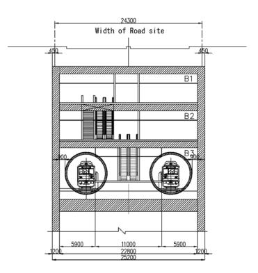
Figure 4.2.18 Cross Section of a Typical Station
