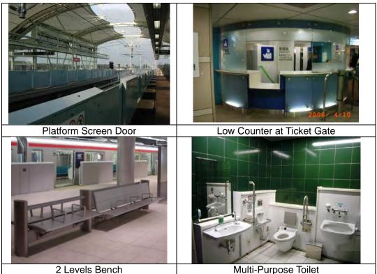
Figure 4.2.58 Barrier Free Design Features
