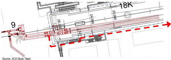
Figure 4.2.55 Detour Plan of Water Pile
