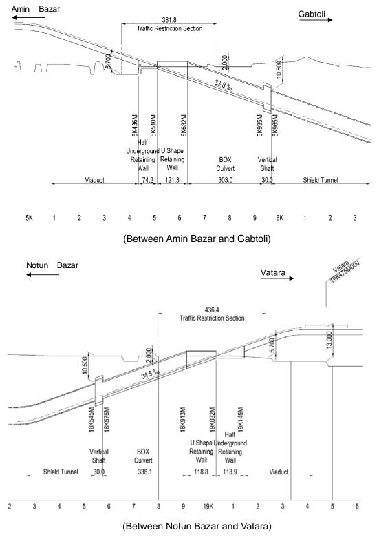
Figure 4.2.9 Detail Profile of Transition Section
