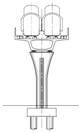
Figure 4.2.1 Standard Cross Section of Pier
