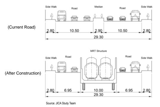
Figure 3.2.13 Cross Section of Road
