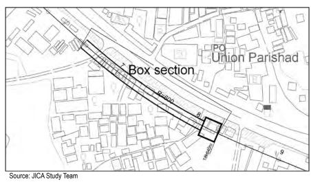
Figure 4.2.27 Location of Launching Shaft (between Amin Bazar Station and Gabtoli Station)
