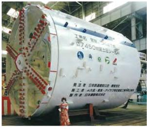
Figure 4.2.24 Reference Photo of Earth Pressure Shield Machine
