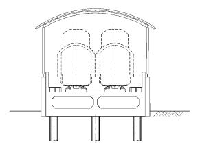
(Half Underground Retaining Wall Section)
