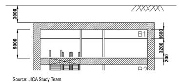
Figure 4.2.39 Case of Shield Machine Transportation Using Ball Sliders
