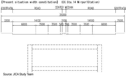
Figure 4.2.40 Current Road Width at Mirpur 14 Station
