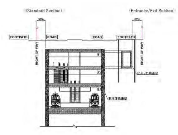
Figure 5.11.3 Typical Cross Section of Underground Station
