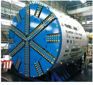
Figure 4.2.26 Reference Photo of Slurry Shield Machine
