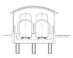
(U Shape Retaining Wall Section)
