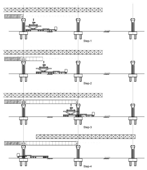
Step 1 : Erection Girder (EG) is in position. 1st precast segment (edge segment) is transported by a long trailer from the construction yard and its position should be just under EG. The segment is hanged by suspension cables with EG and turned by 90 degree and is in placing.
