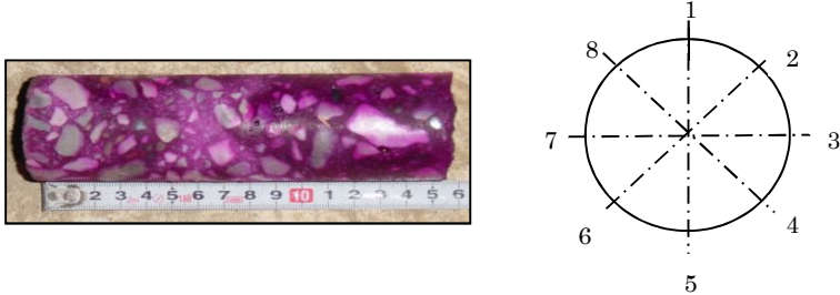
Figure-6.3.5 Estimation of carbonation depth by core extraction
