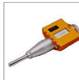
Photo-6.3.2 Schmidt rebound hammer
