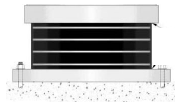
Elastomeric Pad with Steel Plate
