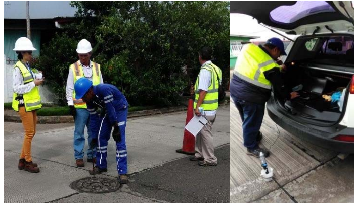
Figure 2.3.17 Investigation of water infiltration with EC meter (sample being analyzed with PC)
