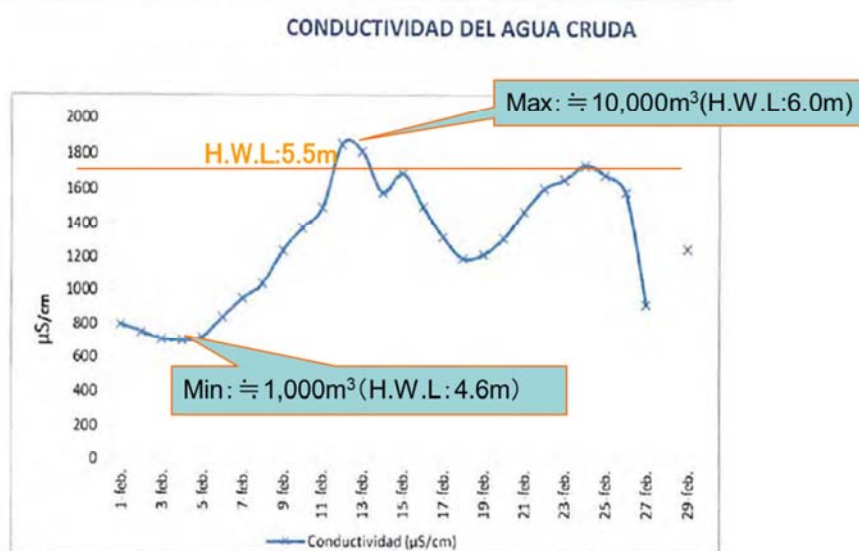
Figure 2.3.19 Relationship between reverse flow of seawater into the sewerage network in JDWWTP (EC values) and Tidal levels
