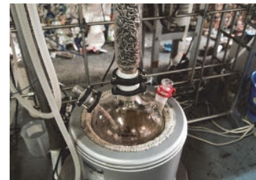
distilling process to refine the ethanol
