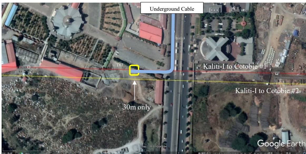
Fig. 7.1-3 Tower plotting for cable termination
