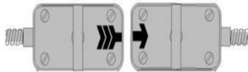
Fasten the transducers the way that the engravings form an arrow.
