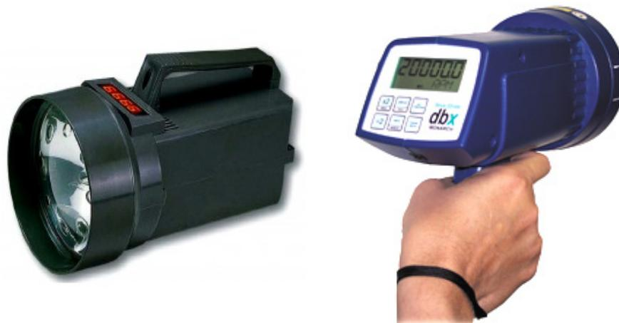
Gambar 12.25 Stroboscope
