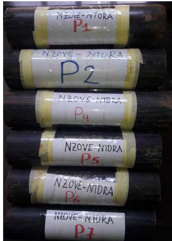
Figure 4: \phi 90 mm undisturbed samples
