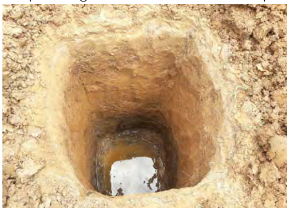
Figure 1: Excavated Trial Pit
