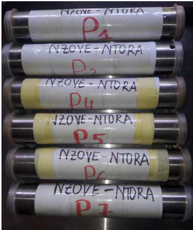
Figure 3: \phi 20 mm, undisturbed samples
