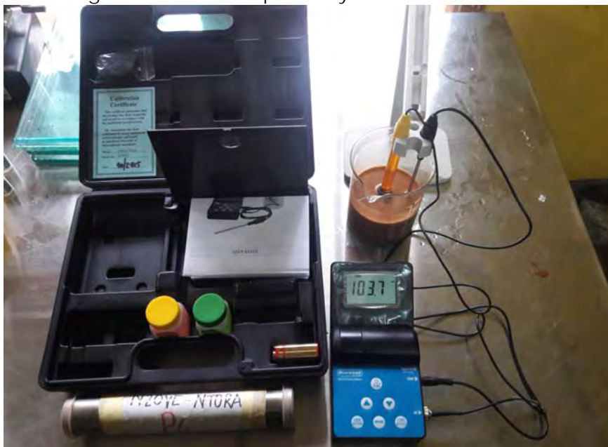
Figure 5: Test arrangement for the electronic method for the determination of soil PH and ORP (BS 1377 -3)
