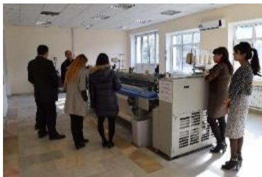
Air jet waving machine procured by Toyota Tsusho (Tashkent Institute of Textile and Light Industry)
