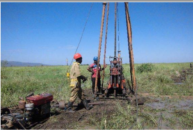
Picture 8. Boring Survey This is the Boring survey to check strength of foundation for Dyke and O&M road. The survey was done at 18 points in total in the area.
