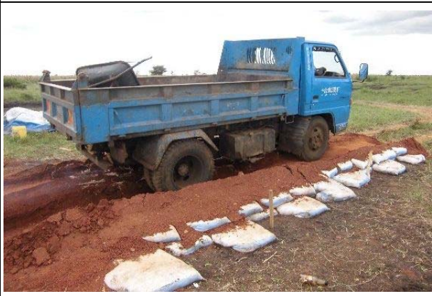
Picture 9. Sand Back Test This is the sand back test to check the strength of them filled with Black Cotton Soil
