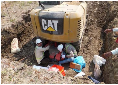
Image-2 Plate Loading Test (The calculation formula for the ultimate bearing capacity was led based on the results of the plate loading test)
