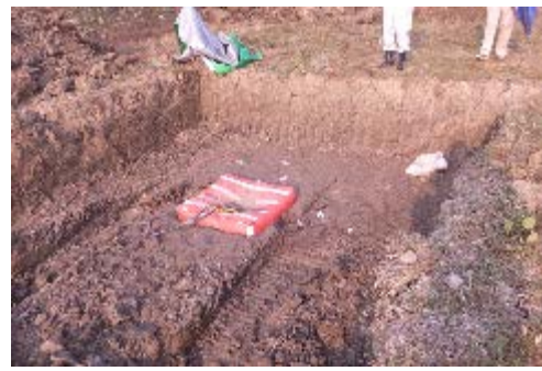
Image-2 Plate Loading Test (The calculation formula for the ultimate bearing capacity was led based on the results of the plate loading test)
