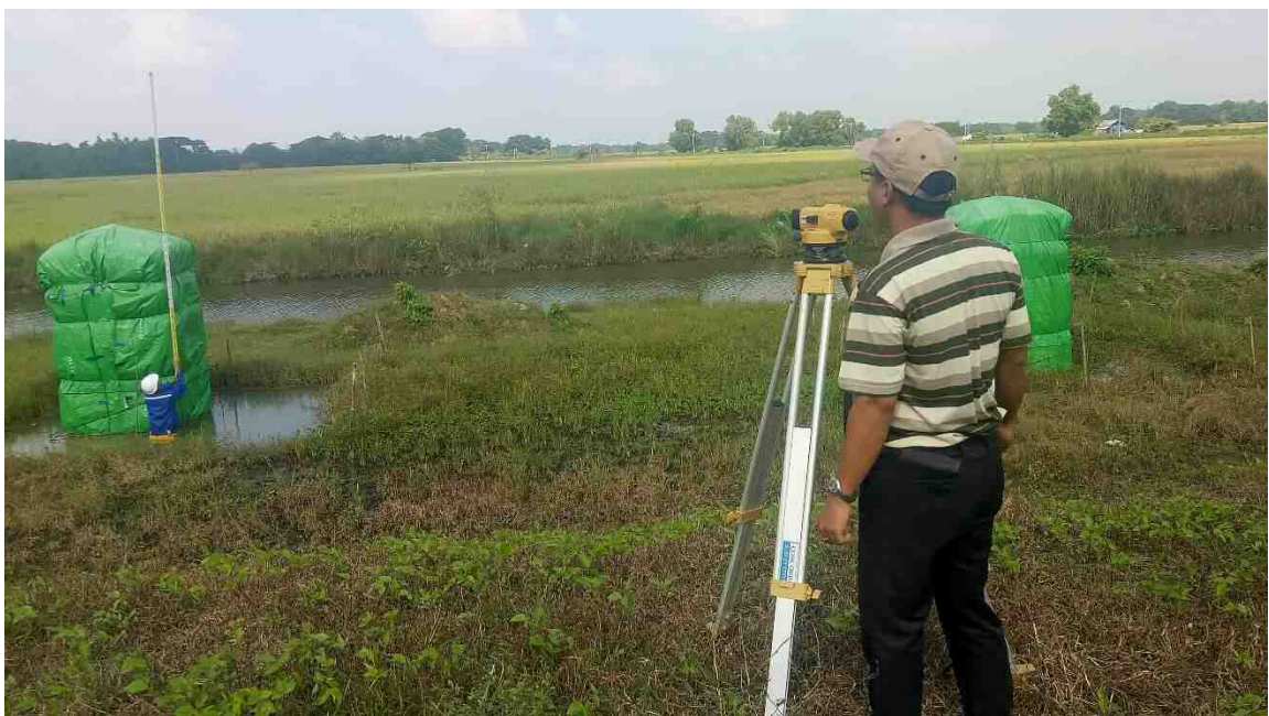
Photo - 2.2 Measurement Condition of Settlement of Loading Test
