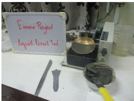
Photo - 4.3 Atterberg Limits Test (Liquid Limit & Plastic Limit)
