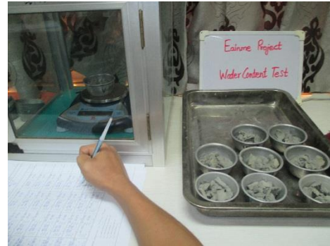
Photo - 4.1 Natural Moisture Content Test
