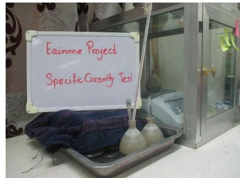
Photo - 4.2 Specific Gravity Test
