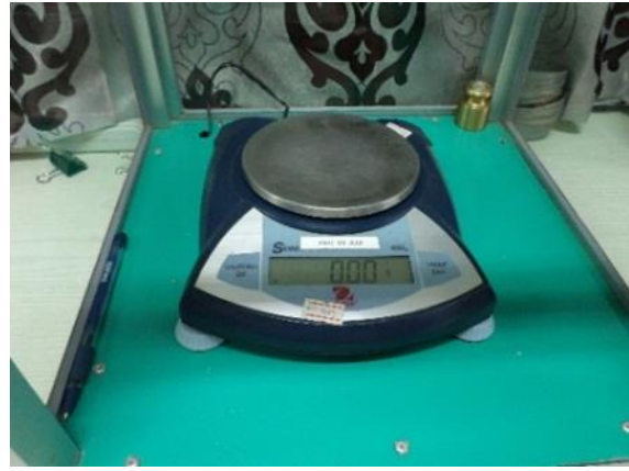
Photo - 1.10 Electrical Balance
