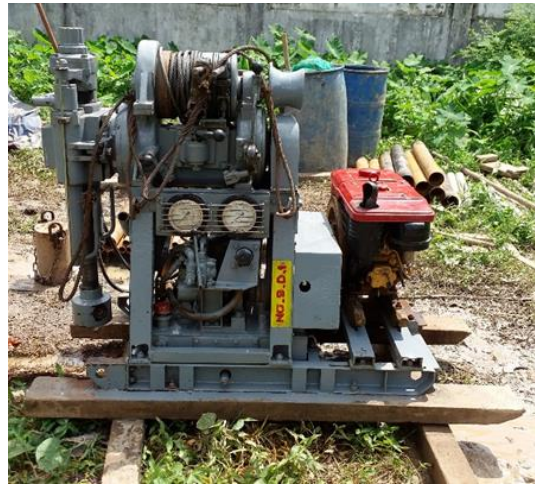
Photo - 1.7 TOHO-D1 Drilling Machine
