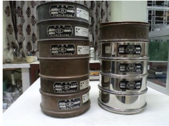
Photo - 1.12 Sieve Test Equipment
