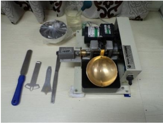
Photo - 1.11 Atterberg Limits Apparatus
