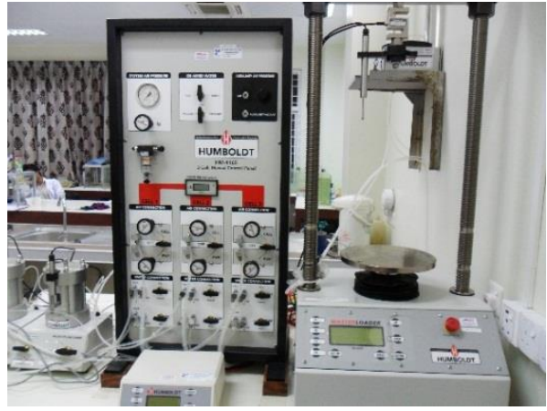
Photo - 1.16 Triaxial Compression Test Machine
