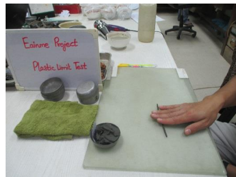
Photo - 4.3 Atterberg Limits Test (Liquid Limit & Plastic Limit)
