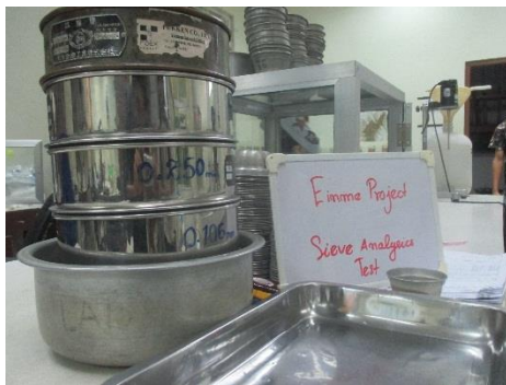
Photo - 4.4 Grain Size Distribution Test
