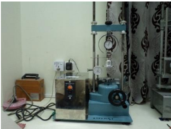
Photo - 1.13 Unconfined Compression Test Machine
