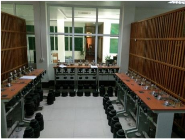
Photo - 1.15 Consolidation Test Apparatus
