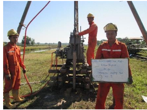
Photo - 3.8 Taking Undisturbed Sampling
