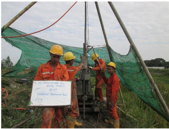
Photo - 3.7 View of Standard Penetration Test and SPT Sample
