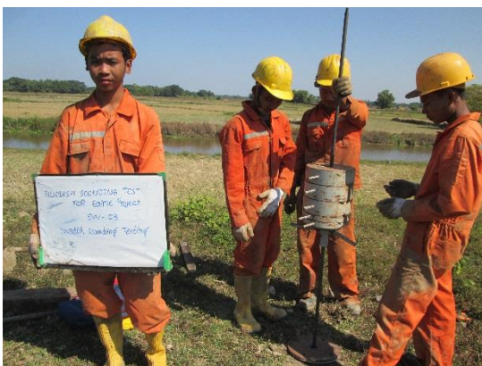
Photo - 1.5 View of Swedish Sounding Test
