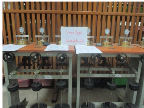
Photo - 4.8 Data reading for one dimensional Consolidation Test Results
