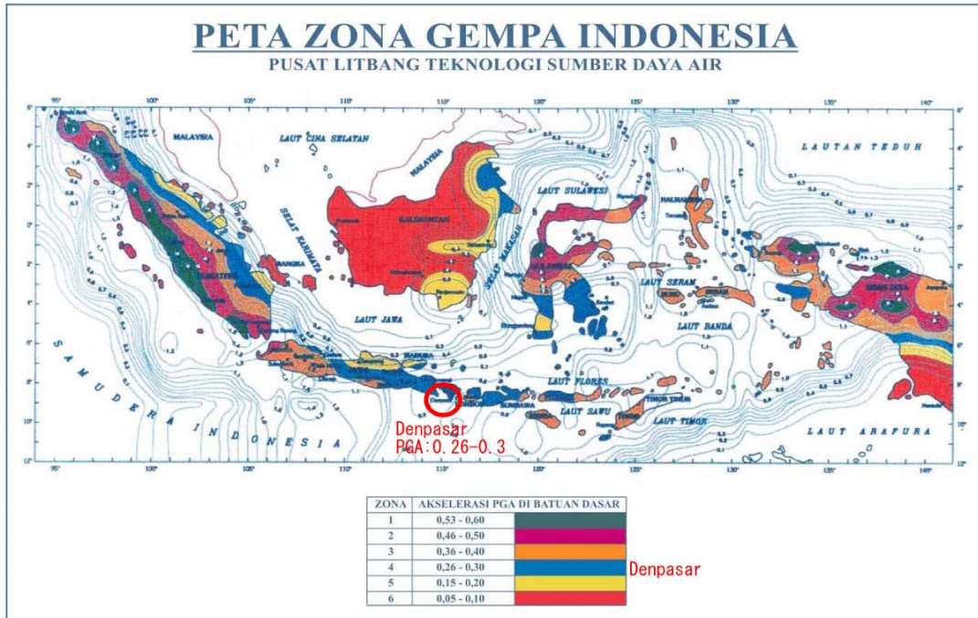
Figure A5.5-1 Design seismic load regulated in bridge seismic design code of Indonesia
