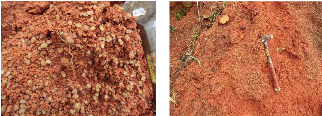
Figure 5.4.1 Weathered Quartz-biotite Granite and Biotite Schist Turning Reddish Brown (White grains in the left photo are quartz)
