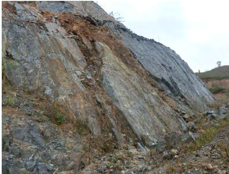
Figure 5.4.7 A dip Slope Structure of Slate and Shale and Slope Failure (at 260 km point of Pre F/S route)
