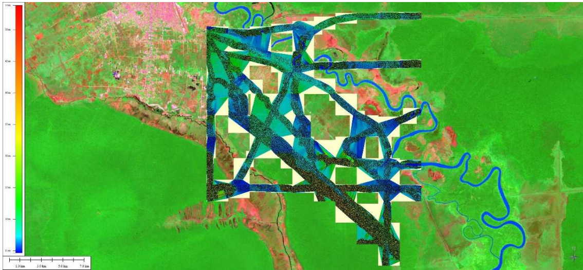
Figure 2-2 LiDAR – DSM and – DTM for Block C as overview .(Projected by Global Mapper: UTM, Zone-49, WGS84, meters)
