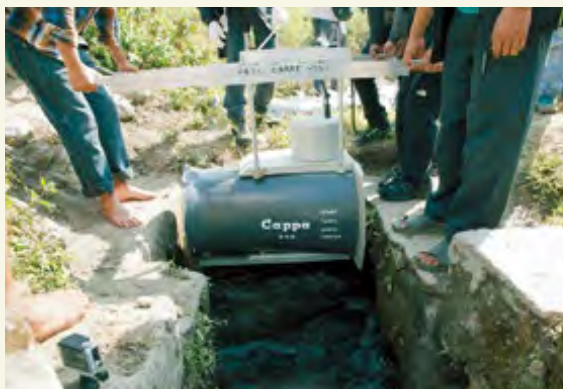
The small hydropower generator Cappa can be carried by two adults
