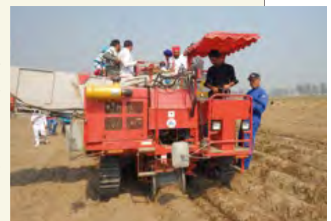
Toyo's self-propelled potato harvester in action
