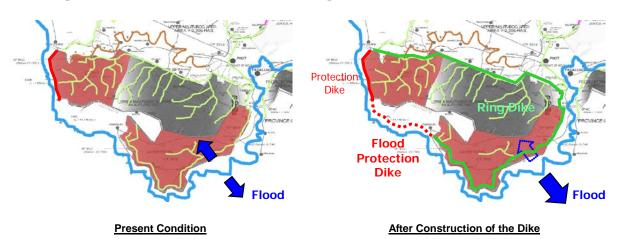
Figure 3.2.6 Image of Flood Situation under Present Condition and After Construction of the Dike Source JICA Survey Team
