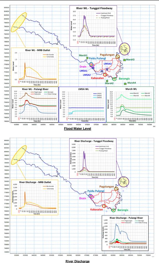
Figure 3.5.17 Flood Water Level and River Discharge (After Construction of the Dike) (Return Period: 50 year) Source: JICA Survey Team
