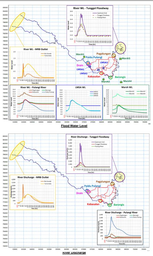
Figure 3.5.12 Flood Water Level and River Discharge (Present Condition) (Return Period: 100 year) Source: JICA Survey Team
