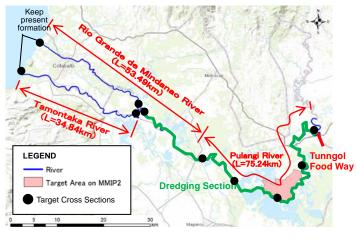
Figure 3.7.1 Dredging Sections and the Target Cross Sections Source: JICA Survey Team
