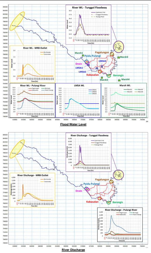
Figure 3.5.11 Flood Water Level and River Discharge (Present Condition) (Return Period: 50 year) Source: JICA Survey Team
