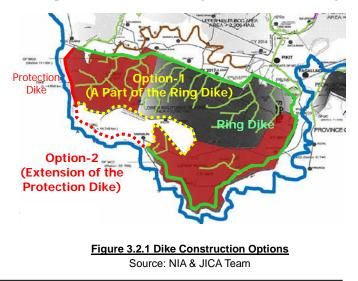
1) high dike reaching over 6 m height would require foundation treatment which causes a surge of the construction cost. Even with the most economical measure of foundation treatment, e.g. sand compaction pile method, additional PhP is required for the treatment. Thus, the EIRR would fall in negative range (-0.2%).
