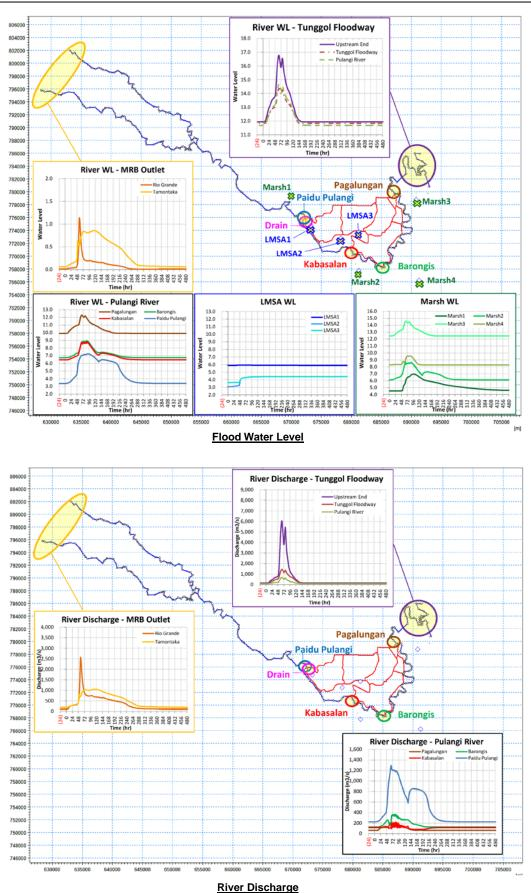
Figure 3.5.16 Flood Water Level and River Discharge (After Construction of the Dike) (Return Period: 30 year) Source: JICA Survey Team
