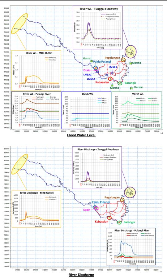
Figure 3.5.13 Flood Water Level and River Discharge (After Construction of the Dike) (Return Period: 2 year) Source: JICA Survey Team
