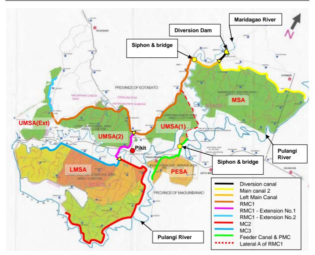
Figure 2.4.3 Irrigation Canal Network in MMIP Source of Base Drawing: NIA- PMO
