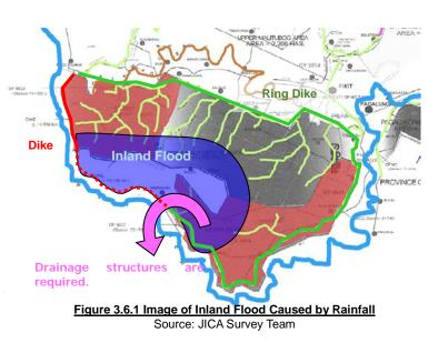
drainage structures are necessary to reduce such inundation area, and to realize the purpose of the dike construction.
