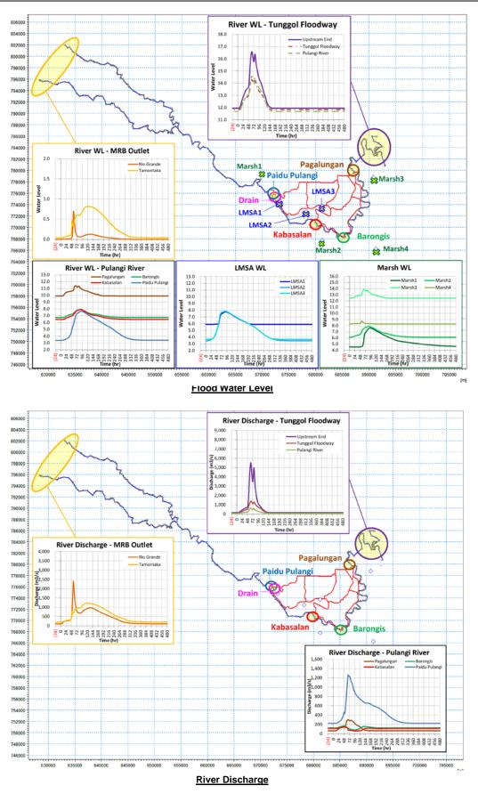
Figure 3.5.9 Flood Water Level and River Discharge (Present Condition) (Return Period: 20 year) Source: JICA Survey Team
