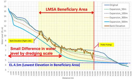
Figure 3.7.3 Longitudinal Profile of the Maximum Flood Water Level Source: JICA Survey Team
