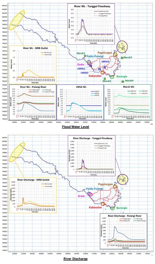
Figure 3.5.7 Flood Water Level and River Discharge (Present Condition) (Return Period: 2 year) Source: JICA Survey Team
