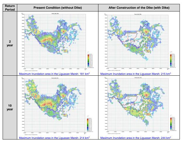
Figure 3.5.3 Simulation Results (Maximum Inundation Area) (1/2) Source: JICA Survey Team
