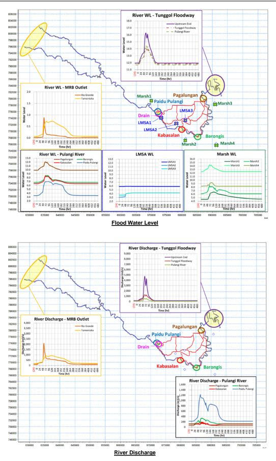
Figure 3.5.14 Flood Water Level and River Discharge (After Construction of the Dike) (Return Period: 10 year) Source: JICA Survey Team
