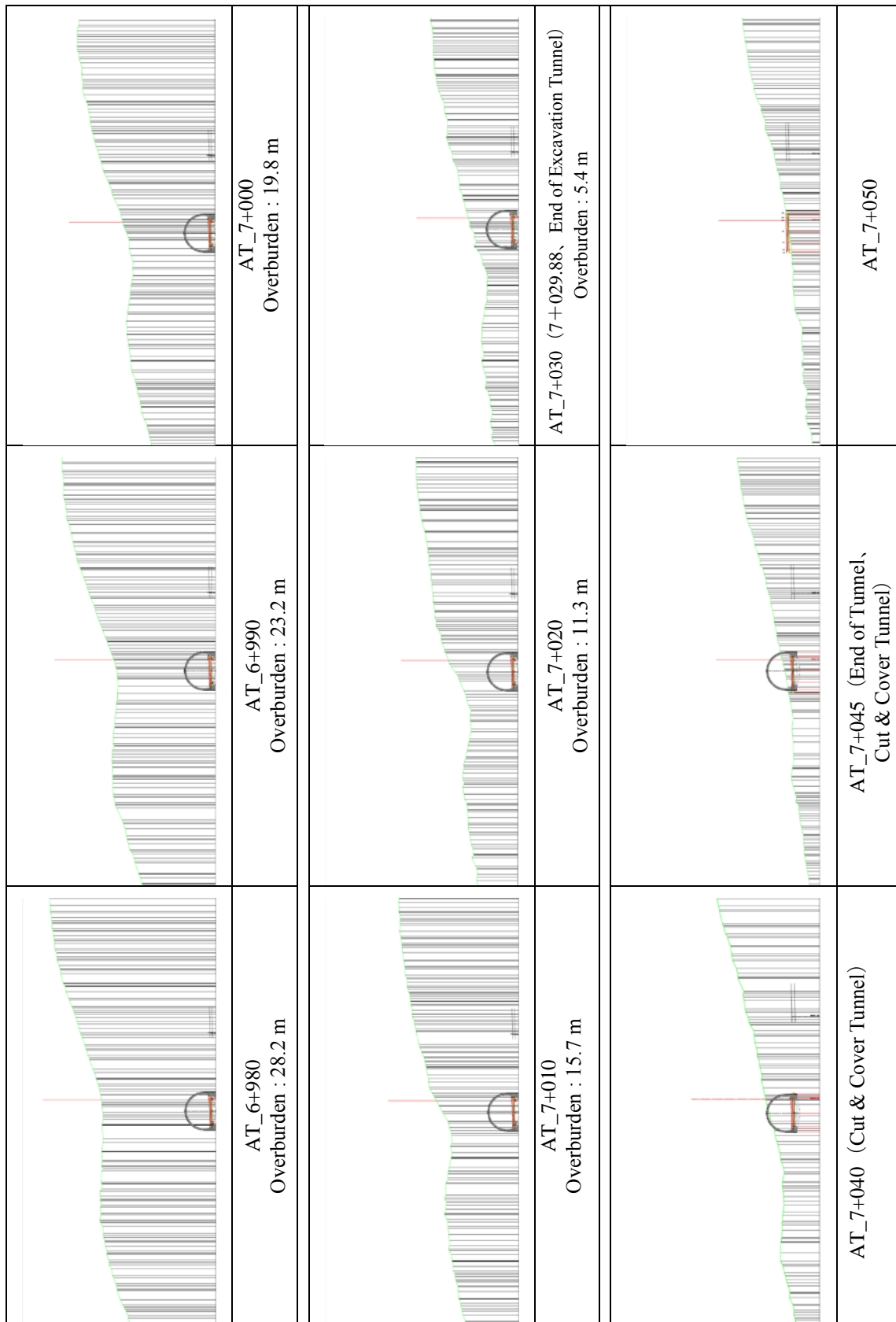
Figure 15: Topography and Tunnel Location in Portal Zone (West) of Tunnel AT-4
