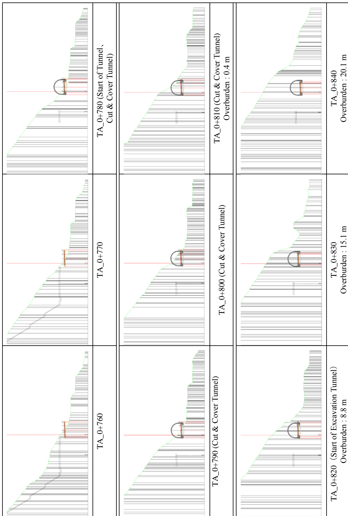
Figure 7: Topography and Tunnel Location in Portal Zone (East) of Tunnel TA-2
