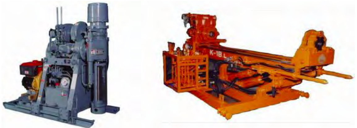
Photo 4.8 Rotary drilling machines: Small type drilling machine (left), horizontal drilling machine (right)
