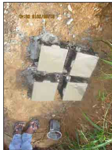
Test cubes cast for testing
