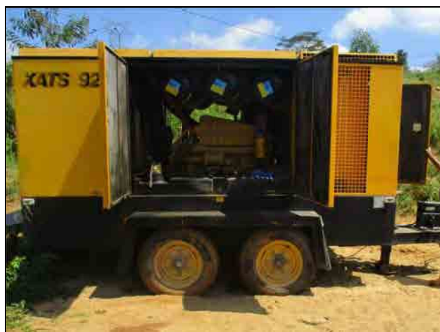
Atlas Copco Compressor stationed at the site
