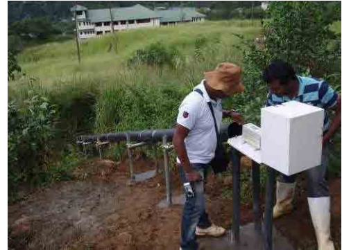
Figure 4.1 Monitoring Survey of Extensometer
