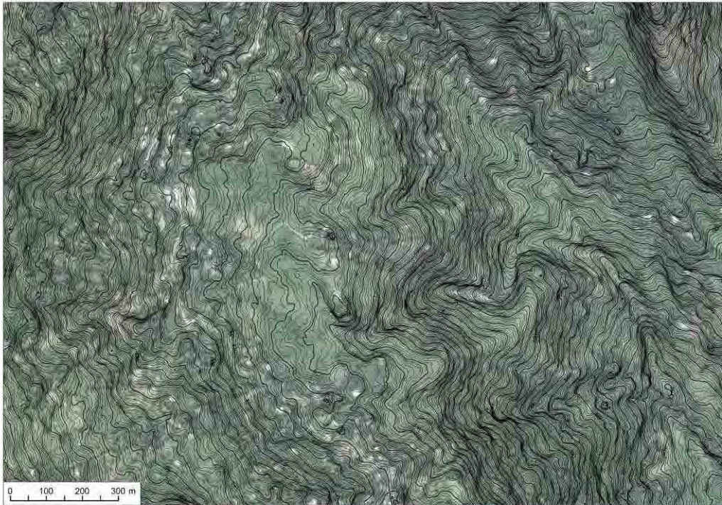
Figure 3.2 DEM Data of Udamadura Site prepared by using UAV
