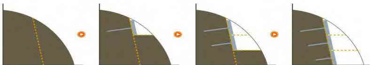
Figure 4.1 Cutting from the top of the slope
