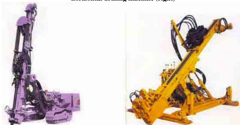
Photo 4.9 Rotary percussion drilling machines: Crawler type (left), skid type (right)
