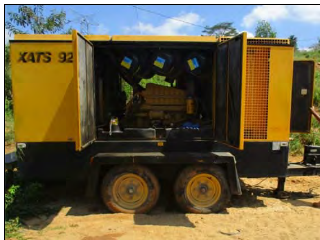
Atlas Copco Compressor stationed at the site
