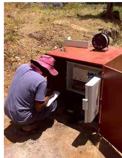
Figure 4.3 Monitoring Survey of Pipe Strain Gauge BN-3
