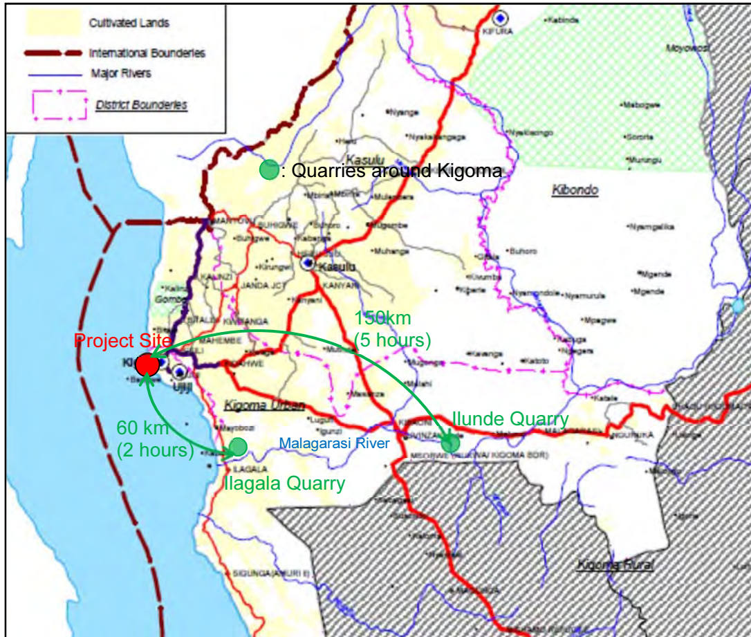
Figure 2.2.4.1-3 Road Conditions in Kigoma and Location of Quarries
