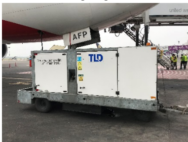
12. Ground Power Unit
