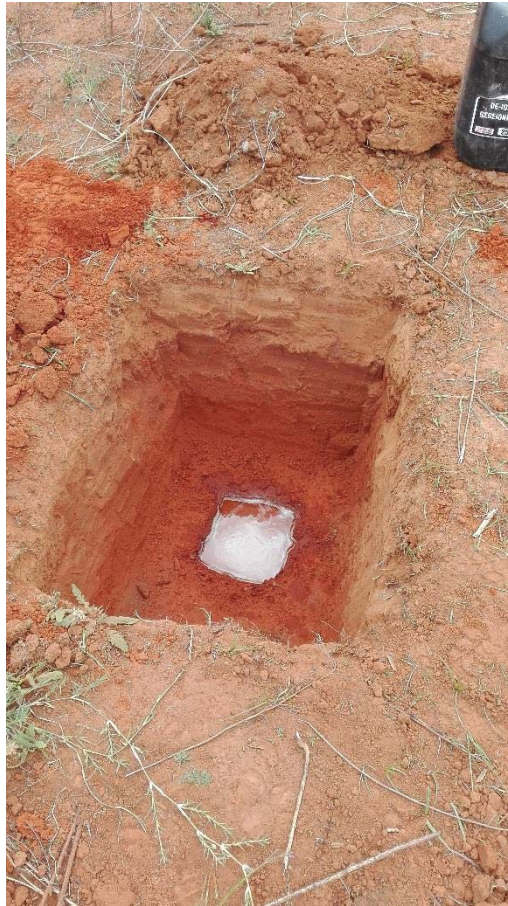
Plate 5 : Percolation testing and subsoils exposed in PT2 pit.
