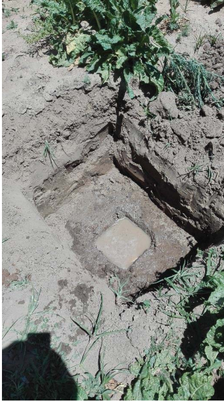
Plate 5 : Soil profile exposed PT1 pit in which percolation test was carried out.
