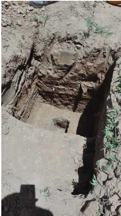
Plate 4 : Soil profiles exposed in TP 1 excavated to 1.5m depth and extended to 2.35m via auger.
