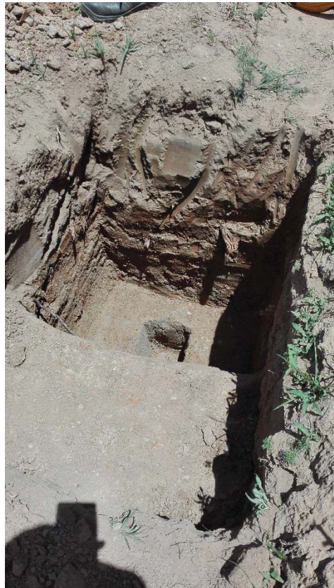
Plate 4 : Soil profiles exposed in TP 1 excavated to 1.5m depth and extended to 2.35m via auger.
