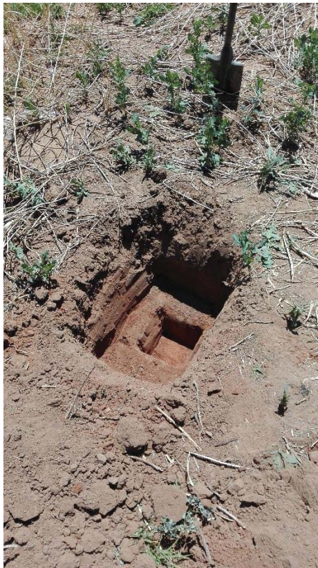
Plate 6 : Soil profile exposed PT2 pit in which percolation test was carried out.
