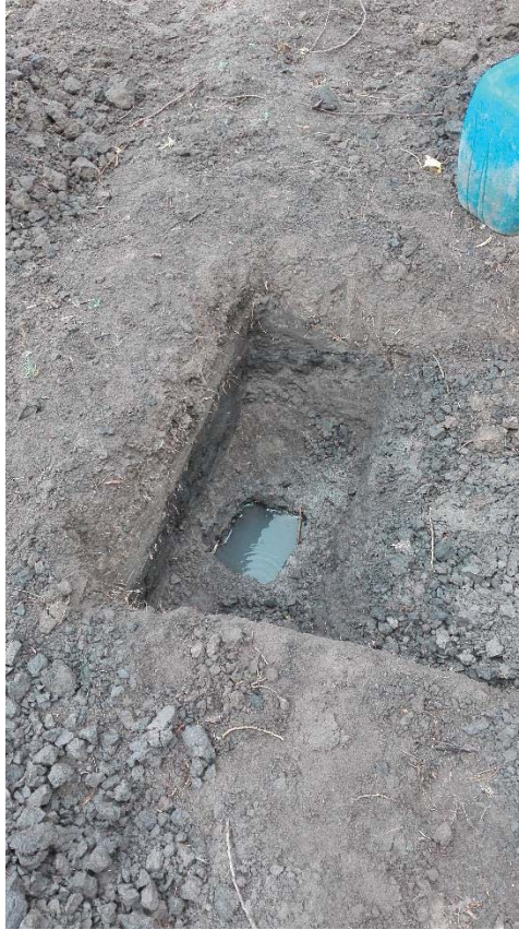
Plate 3 : Typical dark grey clayey subsoils exposed in PT2 pit in which percolation test carried out.
