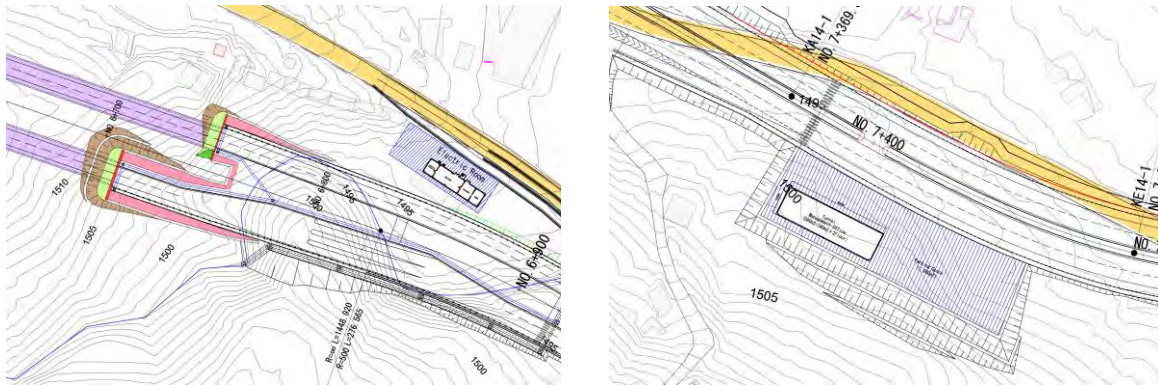
Figure 11.6-12 Layout of Tunnel Management Office and Electric Room (Proposed)
