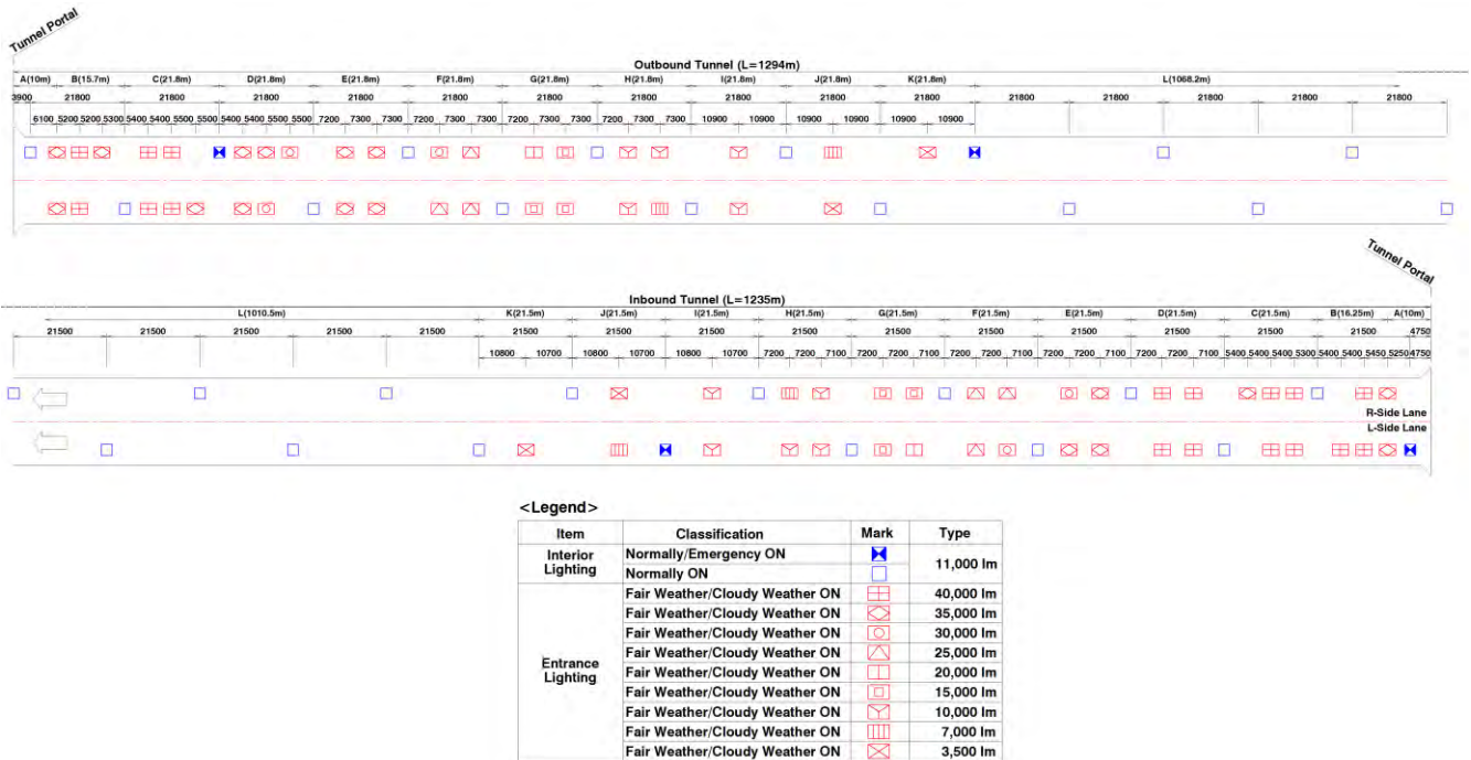
Figure 11.6-3 Layout of Tunnel Lighting
