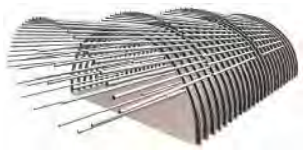
Figure 13.3-1 Non-expansive AGF Method
