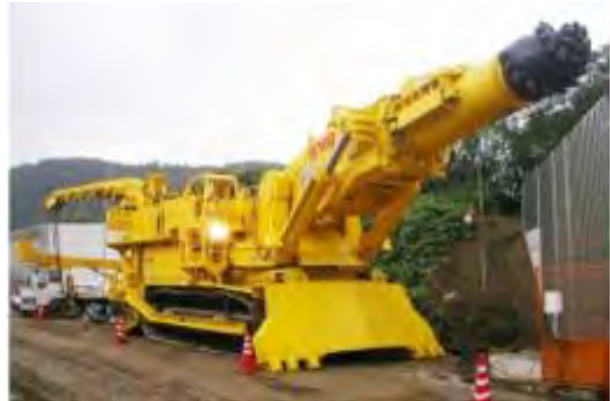
Figure 13.3-3 Hard Rock Excavation Machine
