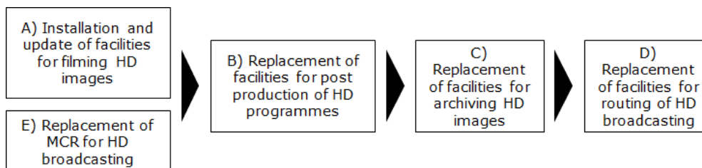
Figure 4.3-2 Flow of upgrade to HD at Broadcasters which have installed MCR for HD broadcasting or started upgrade
