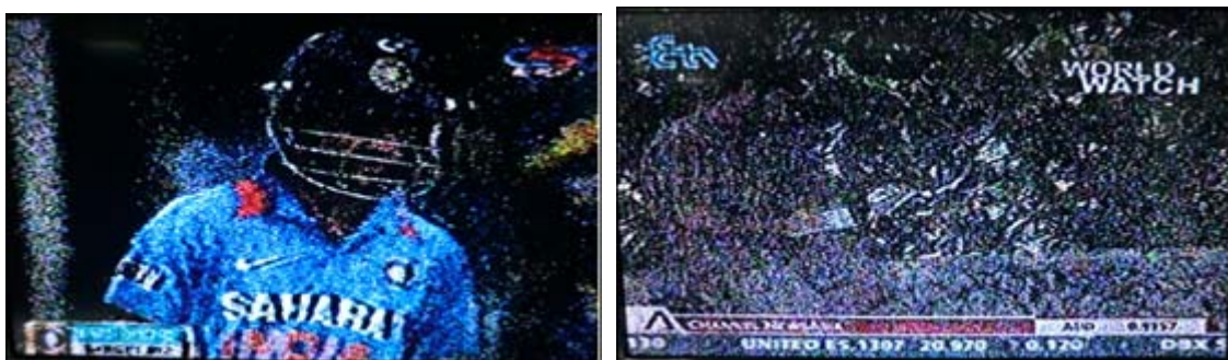
Figure 4.2-1 Example of analogue images received through field strength of about 40dB \mu v/m
